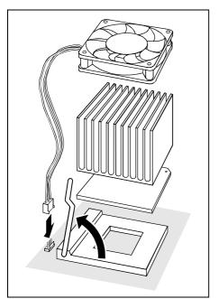
Depending on the configuration variant, you must pull a protective foil off the heat sink or coat the heat sink with heat conducting paste before fitting it.
